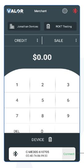
7. Upon detecting the RCKT device, a pop-up window will appear at the bottom of your screen displaying the ID of the RCKT, along with a Connect button. Click on the Connect button, and the Bluetooth icon located on the top right corner of your screen will turn green.
